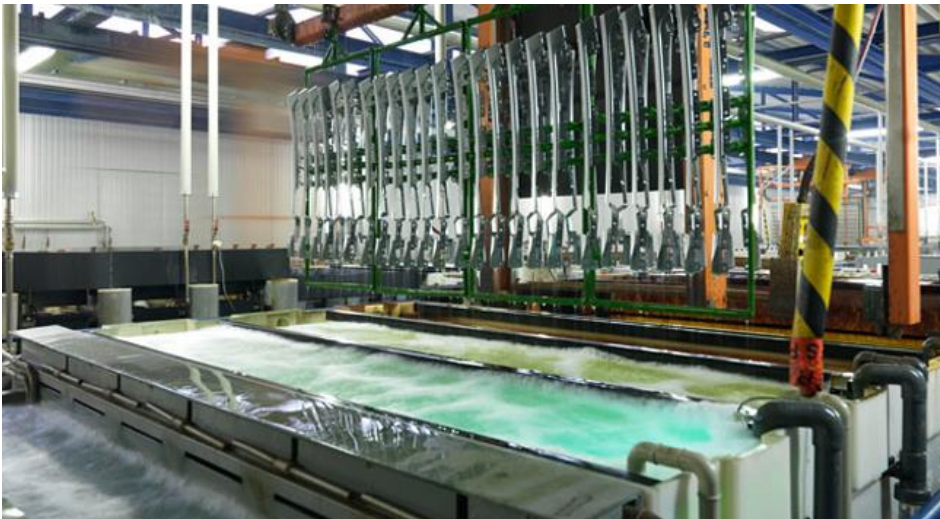
Figure 22: Example of a product carrier loaded on both sides (BIA Kunststoff- und Galvanotechnik GmbH & Co. KG, 2016).
