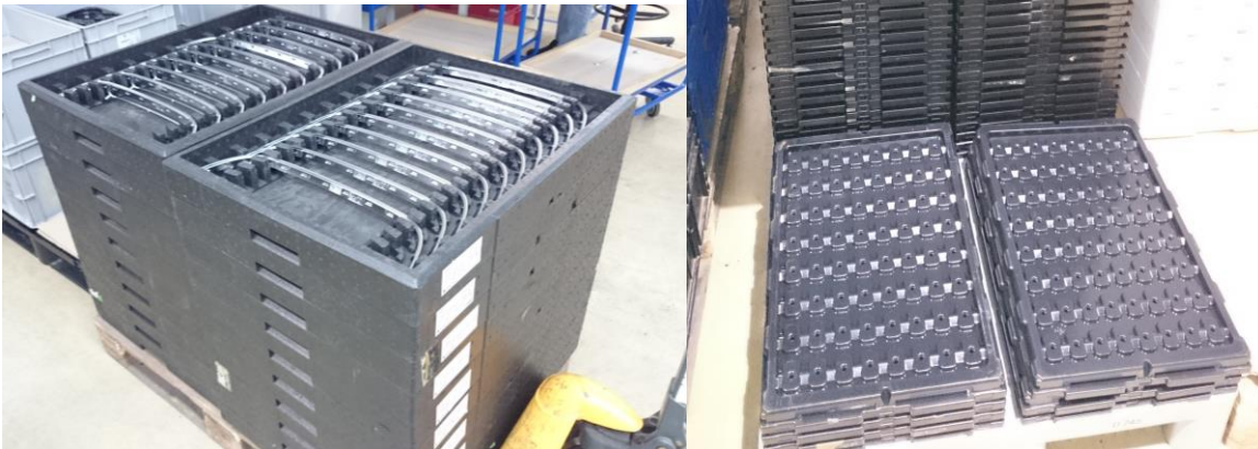
Figure 15: Examples of special containers for chrome treated plastic parts (Fischer GmbH & Co. surface technologies KG, 2016).
