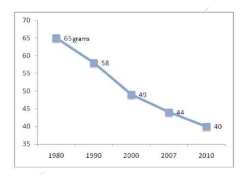
Figure 17: Change in the average weight of a single-use diaper between 1980 and 2010 (Group'Hygiène, 2015)
