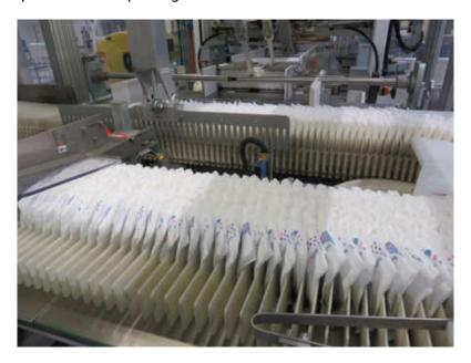
Figure 13: Single-use baby diapers during manufaturing process (Drylock website)
