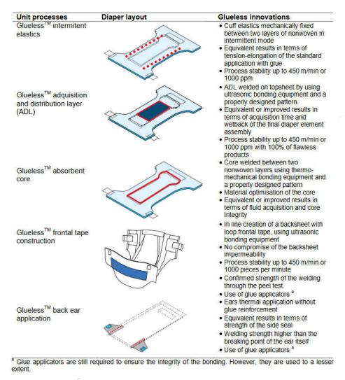
Figure 18: Innovations in the manufacture of glueless baby diapers (based on Fameccanica 2018)
