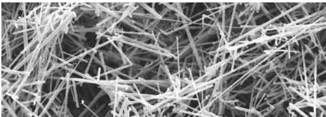
Figure 2: Silar® SC-9M silicon carbide whisker (Source: <http://www.acm-usa.com/silar-sc-9m/>)
