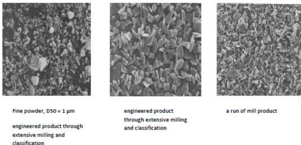
Figure 1: SEM pictures of SiC crude and grains materials (source: SiCMa)
