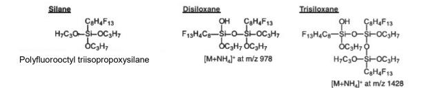
Hydrolysates and condensates identified by ESI/MS (electrospray ionisation/mass spectrometry) spectra of commercial fluorosilane spray products (Nørgaard et al., 2010b)
