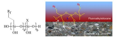
Structural formula and model of a water-based fluoroalkylsilane system. Rf are fluoroalkyl groups and X are hydrophilic groups (Standke et al., year not indicated))
