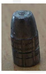
Figure 11 : Tenex 0.22LR lead projectile after travelling through target rifle firearm
