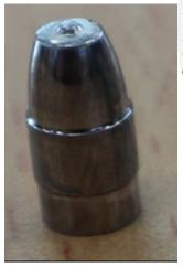
Figure 10 : Original form of Tenex 0.22LR lead projectile
