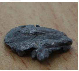
*Figure 12 : Tenex 0.22LR lead projectile after capture in projectile catcher*
