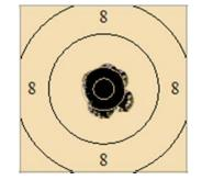
Figure 7: 40 shots of Tenex 0.22LR ammunition lot 1019-06259 on an ISSF 50m Rifle Target
