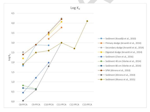
Figure B.4- 4: Trend of Log K<sub>d</sub> with increasing chain length
