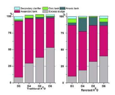
Figure B.3.1 Mean relative fractions of mass loss (%) of D3, D4, D5 and D6 to excess sludge in both the traditional A<sup>2</sup>/O and reversed A<sup>2</sup>/O processes (Xu *et al.*, 2013)
