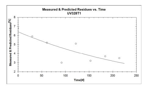
Figure 73: Measured and predicted residues of UV-328 in Treatment 1 vs. time – SFO.
