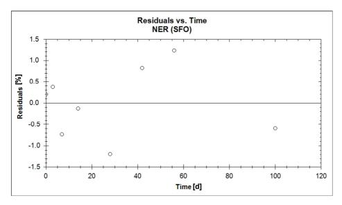
Figure 70: Residuals of NER vs. time in the whole system of an anaerobic pond – SFO.
