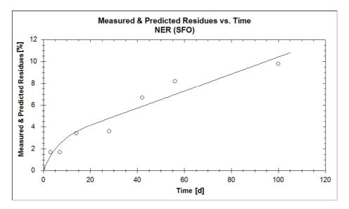
Figure 69: Measured and predicted residues of NER vs. time in the whole system of an anaerobic pond – SFO.
