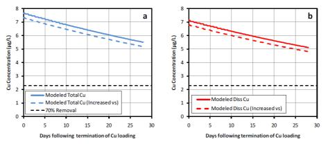
Figure 13. a) Total and b) dissolved copper TICKET-UWM results from post-loading simulations for the observed  $K_D$  and settling velocity scenario. Model simulations use the experimentally-estimated values for the water column  $K_D$  (104.12 L/kg) and settling velocity (0.2 m/d). The blue and red dashed lines refer to simulations with the settling velocity increased to 0.28 m/d. The horizontal black dashed line denotes 70% copper removal.
