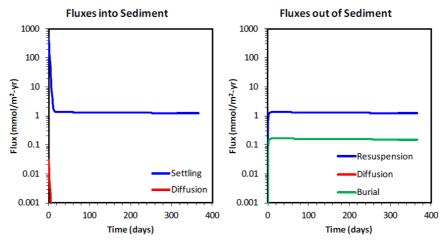
Figure 5. Flux time series plots in anoxic sediment.
