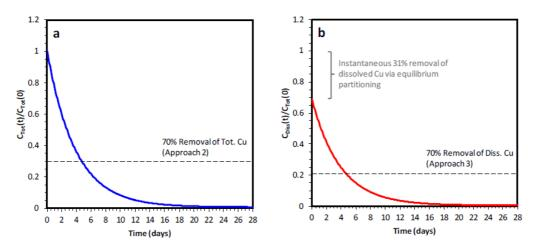
Figure 1. a) Total and b) dissolved copper (Cu) removal from the water column using EUSES model parameters and the linear partitioning method. The initial total copper concentration in the water column, CTot(0), is 35 µg/L. The horizontal dashed lines represents a) CTot(t)/CTot(0) = 0.3 (70% removal of total copper) and b) CDiss(t)/CDiss(0) = 0.3 (70% removal of dissolved copper).
