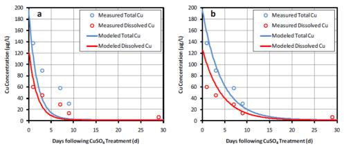
Figure 10. Comparison of TICKET-UWM output (lines) and measured data (points) for copper in the water column of the Saint Germain les Belles Reservoir: EUSES scenario. Model results are from a) the EUSES scenario (water column  $K_D \ 10^{4.48} \ L/kg$ ; sediment  $K_D = 10^{4.39} \ L/kg$ , and settling velocity = 2.5 m/d) and b) the EUSES scenario with the settling velocity reduced to 1.02 m/d.
