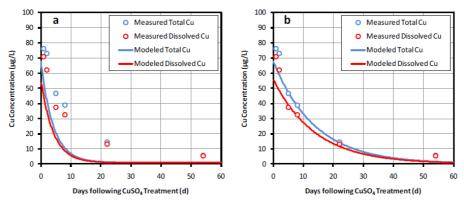
Figure 9. Comparison of TICKET-UWM output (lines) and measured data (points) for copper in the water column of Lake Courtille: EUSES scenario. Model results are from a) the EUSES scenario (water column  $K_D \ 10^{4.48}$  L/kg; sediment  $K_D = 10^{4.39}$  L/kg, and settling velocity = 2.5 m/d) and b) the EUSES scenario with the settling velocity reduced to 0.70 m/d.
