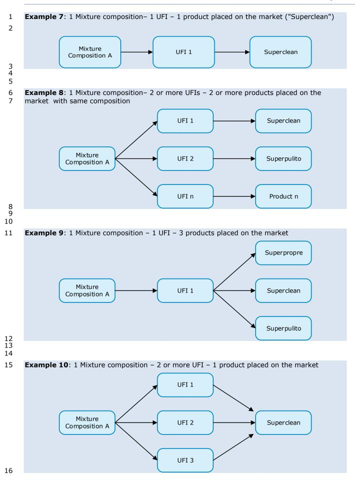
Note to examples 7 to 9: When several UFIs have been generated and assigned to one mixture, all those UFIs need to be included in the submission to the relevant Member State and can be submitted individually or in the same submission. When more than one UFI is assigned to the same product (containing the same mixture), it is sufficient to include only one UFI on the label of the product (example 9) while all UFIs should be indicated on the SDS.
