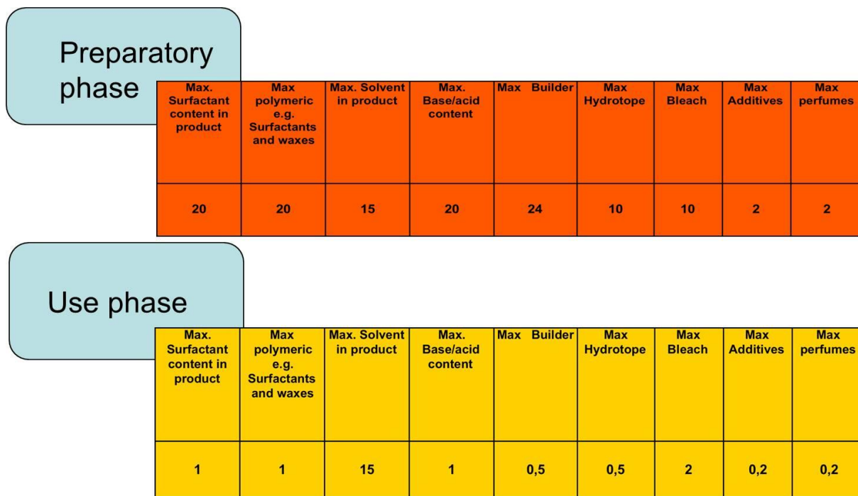
Figure 3a: Example of a cleaning product: Maximum concentration of the ingredients (in weight percentage) during the preparatory and use phases, specified by ingredient type.
