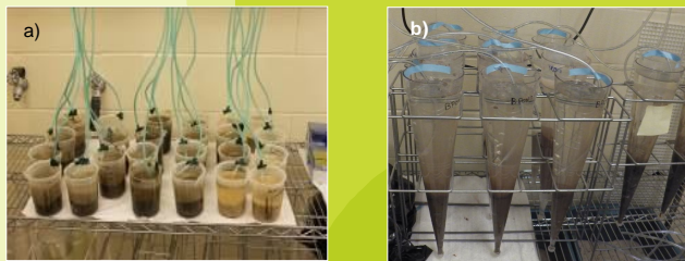
Fig 1. Lab testing set-up for a) C. dilutus and b) fathead minnow sediment toxicity testing.
