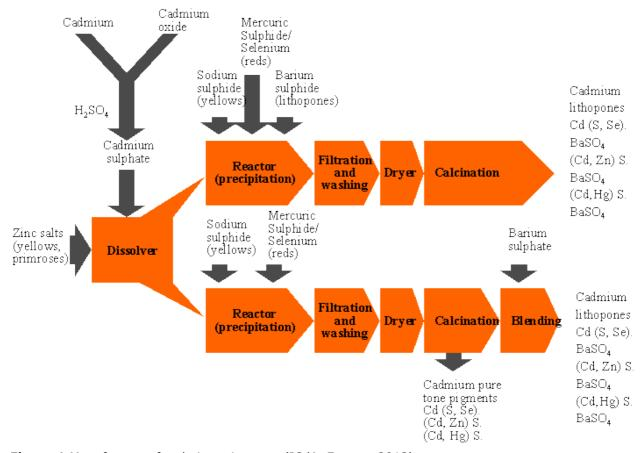
Figure 1 Manufacture of cadmium pigments (ICdA, Europe, 2013)
