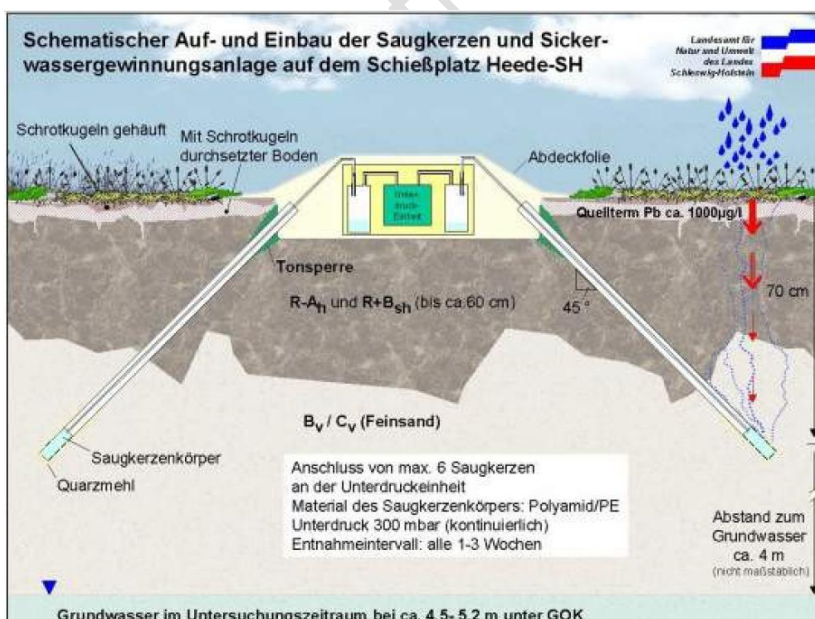
Figure 1-12 Example for measurement of seepage water in a shooting range (LANU, 2005)
