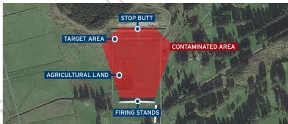
Figure 1-18 Example of lead deposition on agricultural land from a rifle/ pistol range (Australian EPA, 2019)
