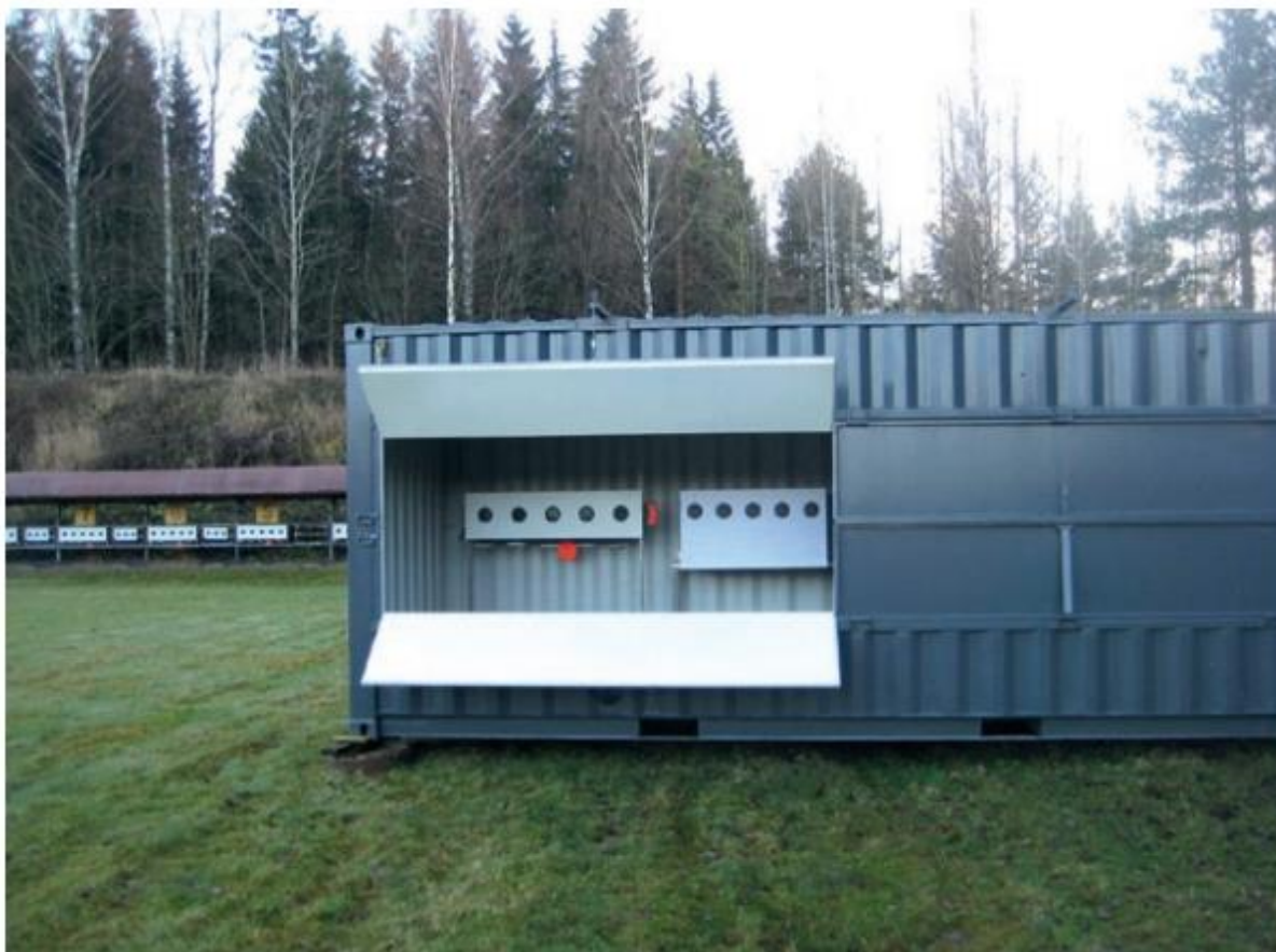
Figure 1-9 Example of a prototype of biathlon target equipment and bullet traps installed in a shipping container (Kajander and Parri, 2014)
