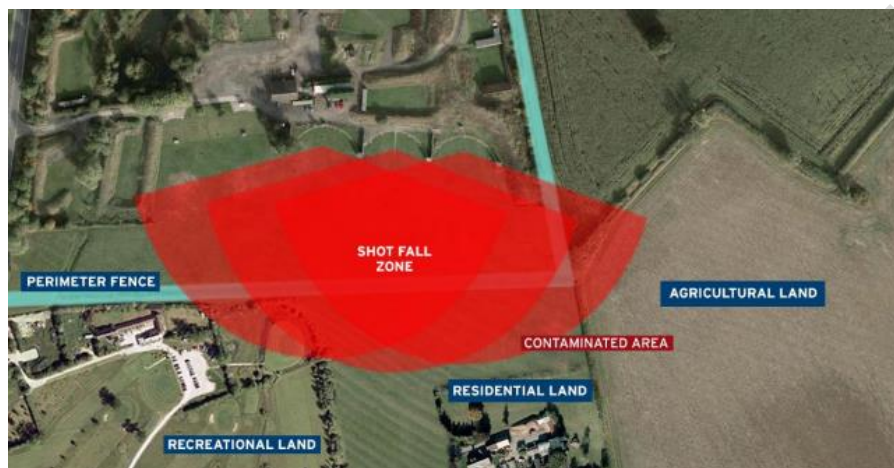
Figure 1-17 Example of lead shot deposition from a shotgun range on lands with different zoning (Australian EPA, 2019)
