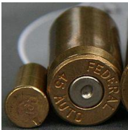
Figure 2-5: calibre markings on the bottom side of a cartridge case and the bottom side of a rimfire cartridge (left) and a centrefire cartridge (right) show in for centrefire the place of the detonator in the centre of the bottom side of a cartridge.
