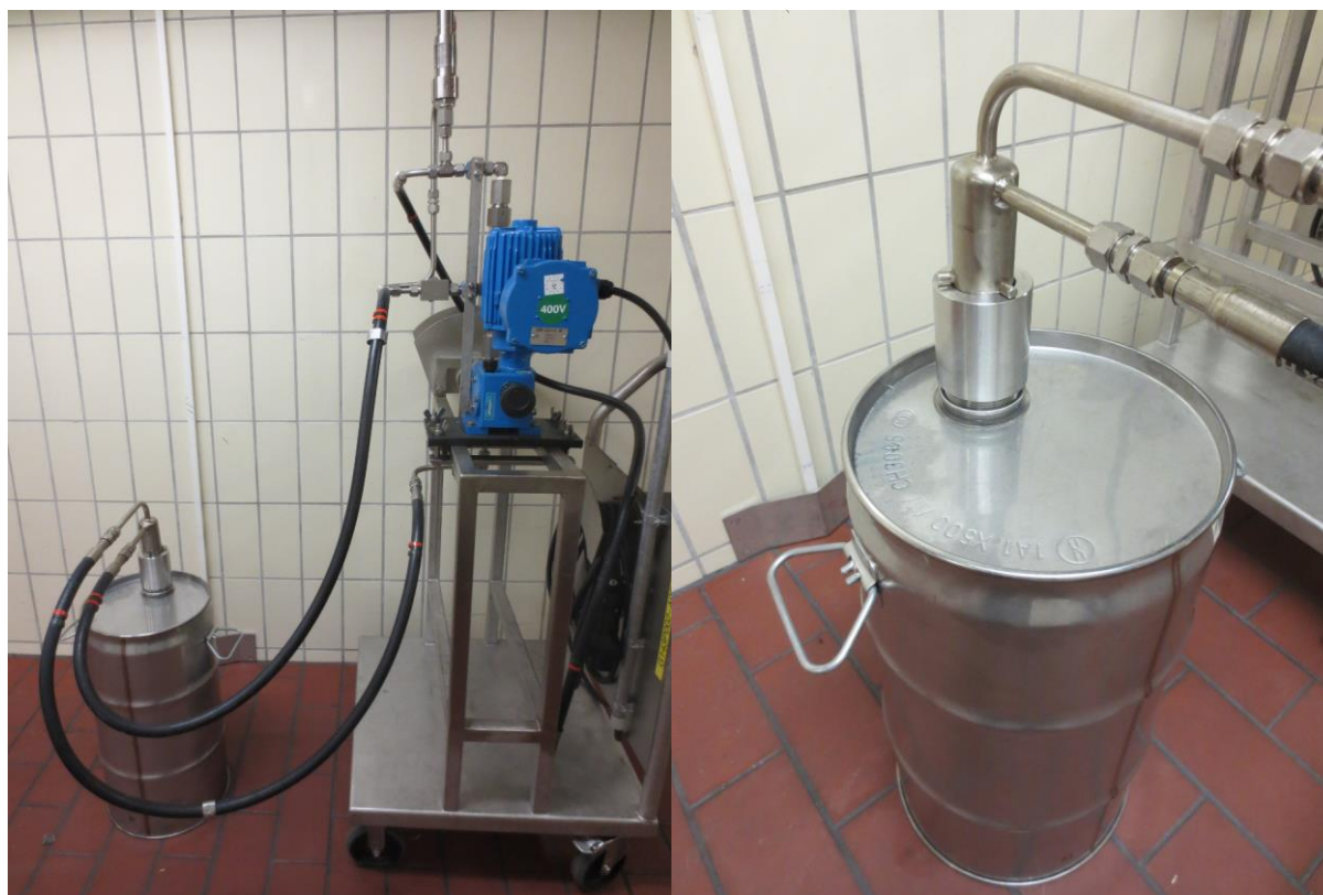
Figure 5: Dosing of the [REDACTED] (reaction mixture) into the reaction chamber by a semi-automatic pump.
