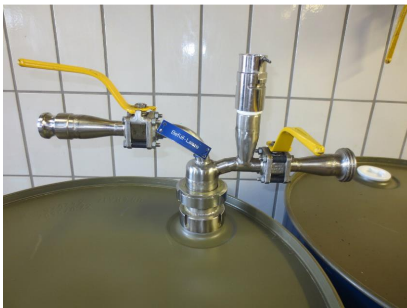
Figure 6: Airtight connections between the 200 L barrel and the centrifuge
