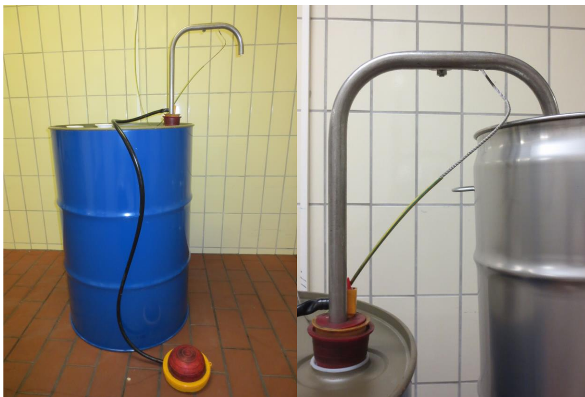
Figure 4: Transfer from 200 L barrel to 30 L barrel for the [REDACTED] (reaction mixture) (diglyme and water).
