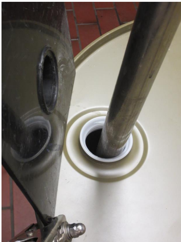
Figure 3: Charging of diglyme from a 200 L barrel into the reaction chamber via a lance.
